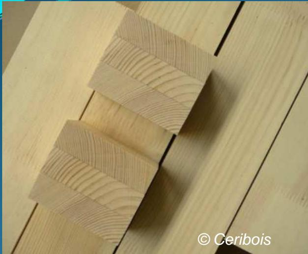
**Fabrication de carrelets 3 plis (L= 3m ; 72 x 86 mm)**
