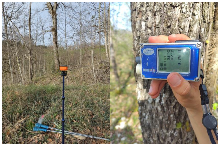
Foto 6 and 7: Deployment of the Hypsometer Vertex in the field, left receiver, right Vertex. Fotos: Sophie Poppe, 2024.
