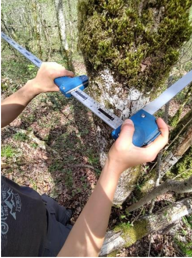
Foto 5: Deployment of tree caliper in the field. Foto: Marie Sallebert, 2024.
